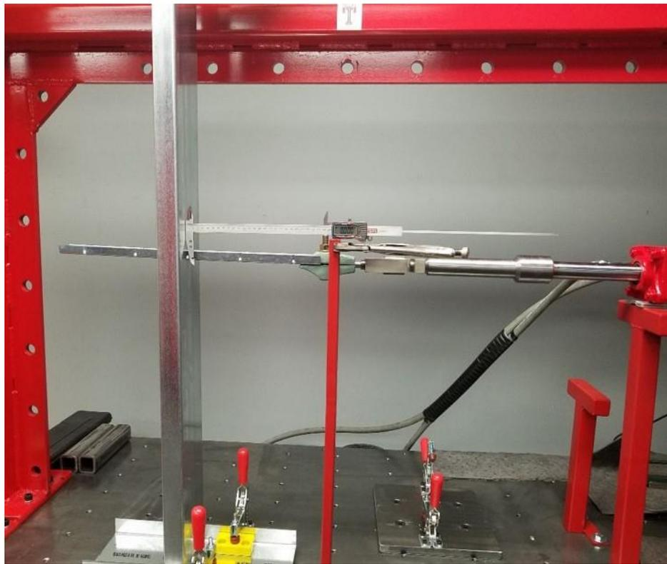
**Figure 5-1: Photograph of the Lateral Loading Test Set-Up**
