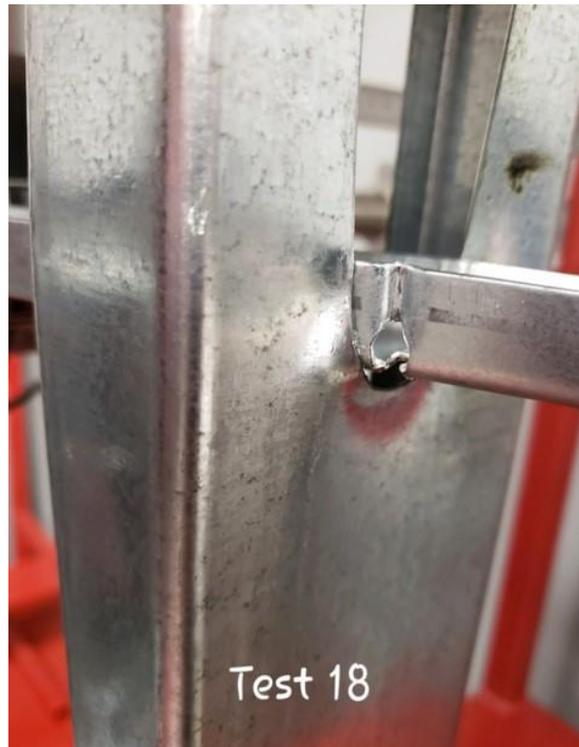
**Figure 6-2: Photograph of Failure Mode for Rotational Loading**
