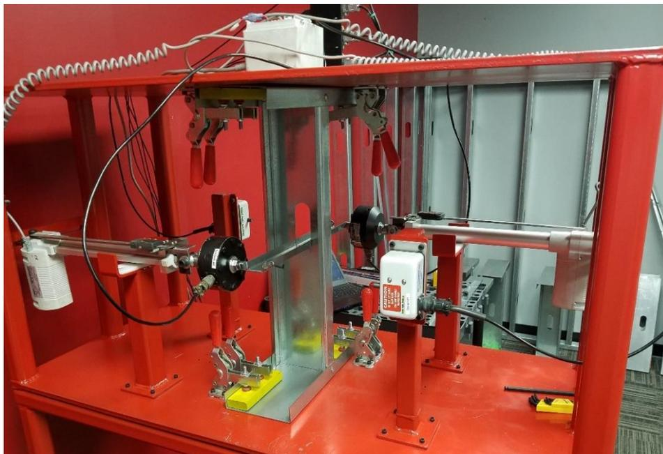
**Figure 5-2: Photograph of the Rotational Loading Test Set-Up**
