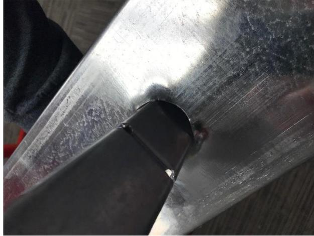
**Figure 6-1: Photograph of Failure Mode for Lateral Loading**
